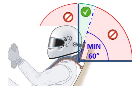
Fig. 2 - Correct collar angle for HANS® device
