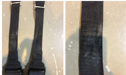
Fig. 31 – Shoulder belts stretched after a severe crash
