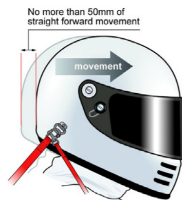
Fig. 9 - Movement to define the tether adjustment
