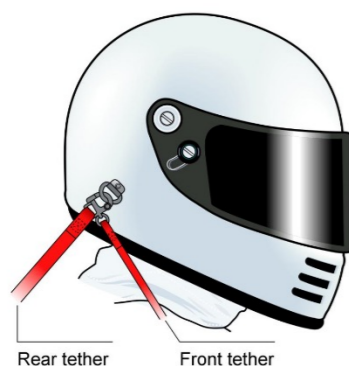
Fig. 8 - Identification of the Hybrid device's tethers
