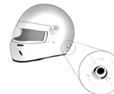
Figure 14 – Damaged M6 terminal
