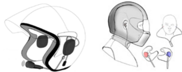
Figure 1 – Helmet-mounted radio speakers vs earplug type transducers
